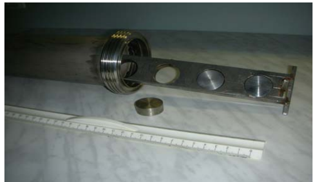
Figure 1 A coupon holder containing two coupons used for biofilm collection
