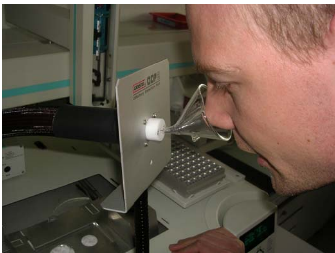
Figure 1 Analysis of T&O compounds at the olfactory detector port (ODP) performed simultaneously with GCMS detection
